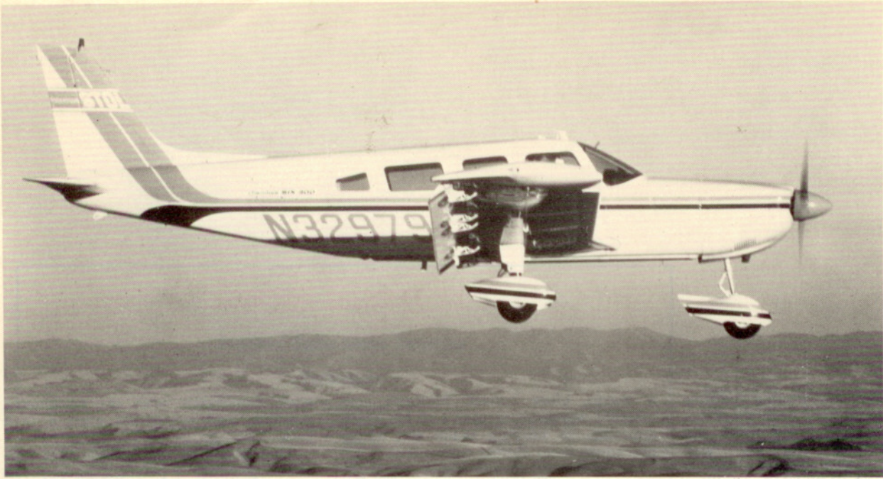
Robertson Cherokee Six lands 205 feet shorter, takes off 350 feet shorter over a 50-foot obstacle, yet cruises 3 mph faster than unmodified version. Conversion costs $8,500.
